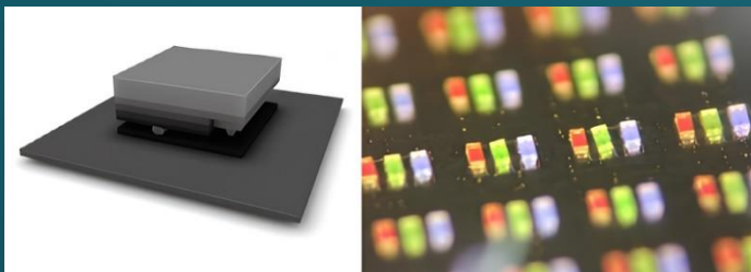
COB fully flip chip design
